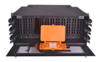
The ODF frame is loaded with adapter module cassettes. One adapter module cassette can be 12cores or 24cores and and is suitable for FC, SC, ST, LC, etc. adapters. 12pcs module cassettes cable be installed. The maximum fiber core is 144 or 288cores for our 3U rack mounted ODF box. It is easy to operate and maintain. The ODF box is widely used in distribution and end connection of indoor cables.
